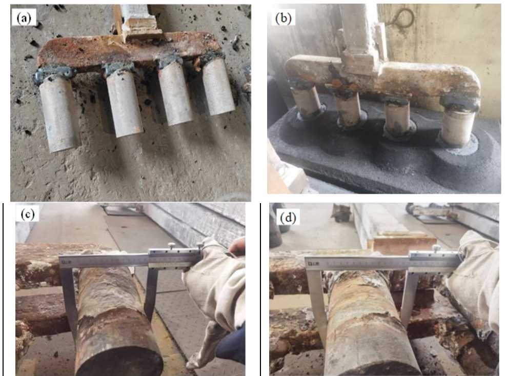
Figure 12. Industrial application scenarios. (a) Welding of oxidation-resistant stubs. (b) Casting of oxidation-resistant stubs. (c) Wear condition of conventional stubs. (d) Wear condition of oxidation-resistant stubs.
