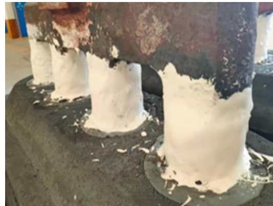
Figure 2. Application of anti-oxidation coating.
